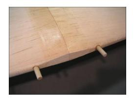
The holes for the wing bolts should be centered fore and aft on the wing bolt plates and spaced 5/8" from the wing center on each side. Mark the holes accurately, then drill all the way through the wing and the plywood wing
