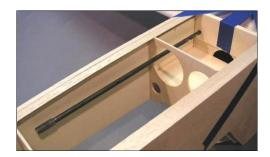
Drill 1/4" holes for the wing dowels into the wing through the holes in F-5. This, I admit, is easier said than done. I ended up using a long drill bit and twisting it by hand. A short piece of fuel tubing slipped over the end gave a better grip. After drilling about an inch on each side, I removed the wing and finished the holes with a power drill.
